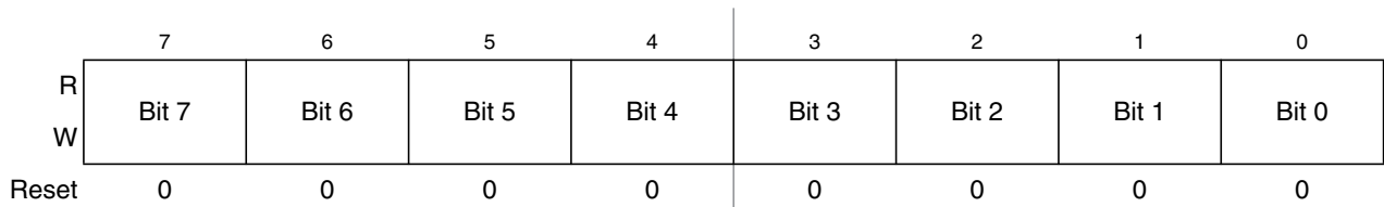
Figure 22-23. Timer Input Capture/Output Compare Register x Low (TCxL)
