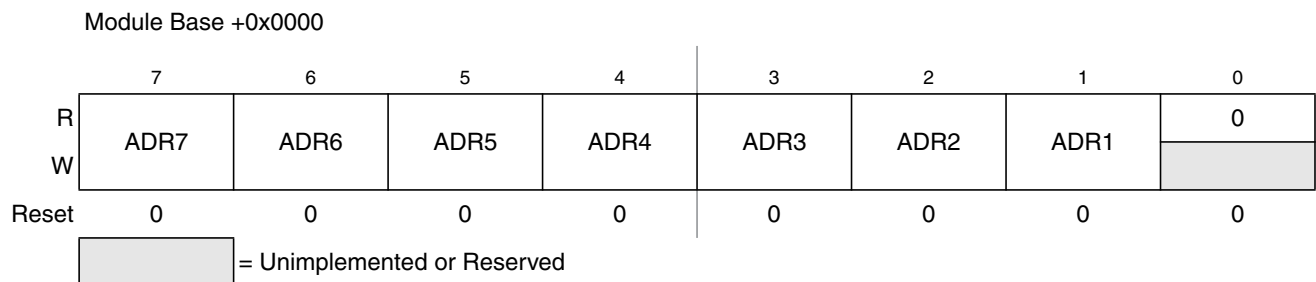
Figure 15-3. IIC Bus Address Register (IBAD)
