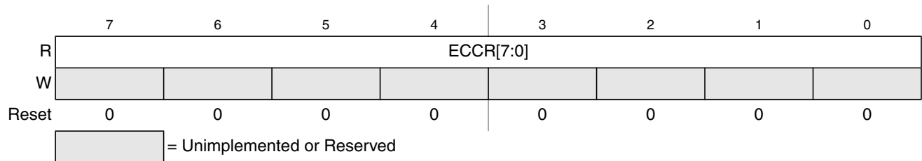
Figure 27-21. Flash ECC Error Results Low Register (FECCRLO)
