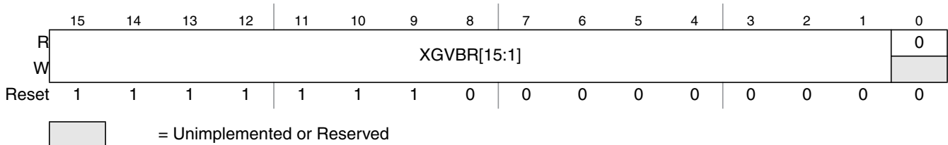
Figure 10-9. XGATE Vector Base Address Register (XGVBR)
