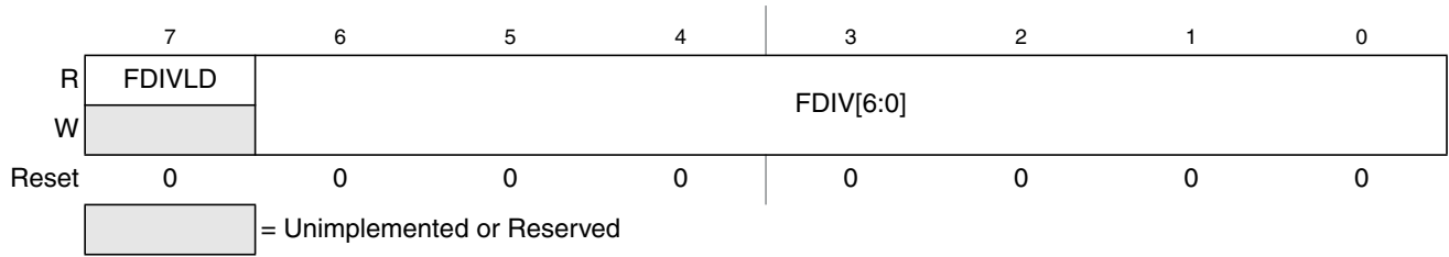
Figure 29-5. Flash Clock Divider Register (FCLKDIV)
