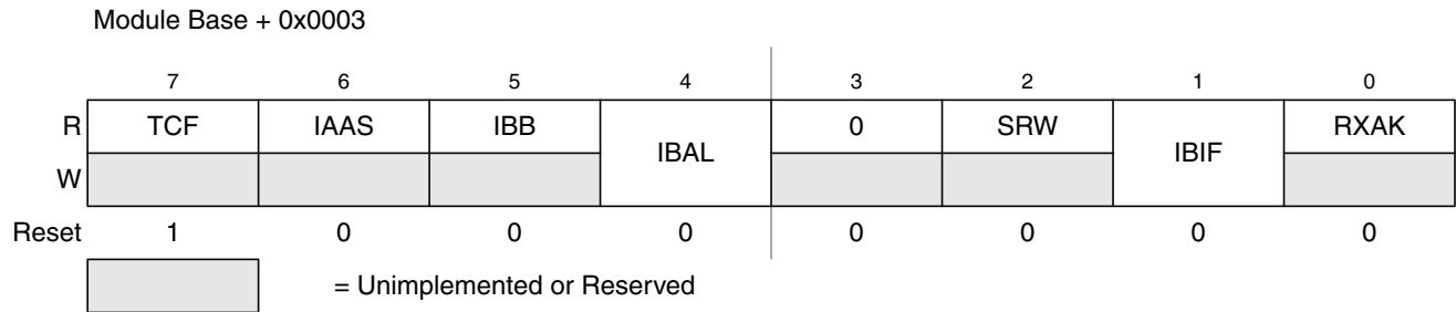
Figure 15-7. IIC Bus Status Register (IBSR)
