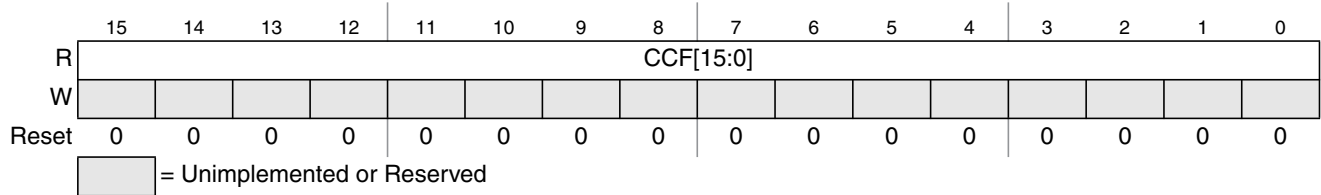
Figure 13-11. ATD Status Register 2 (ATDSTAT2)
